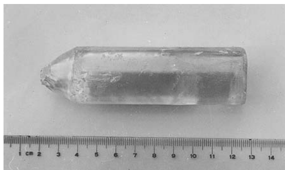
Fig. 2 \text{PbMoO}_4 crystal grown by modified Bridgman method
